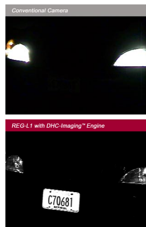
The DHC-Imaging™ technology in REG-L1 captures plates from vehicles moving at up to 100mph under any lighting conditions including highbeam headlight glare.
