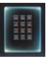
50% intensity; once a key is pressed, the LEDs illuminate at 100% intensity for a period of two minutes. The other high visibility component is a 2 line by 16 character transflective, backlit
